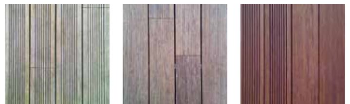
Surface of MOSO® Bamboo X-treme® with different maintenance and cleaning scenarios: weathered, dirty decking (left), weathered, cleaned decking (middle), and re-oiled decking (right).
